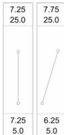
Figure 12: Fluctuation in flow rates across inlet and outlet results in a rotated line (right) and destroys the emergent feature of a vertical line (left).
