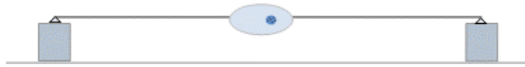
Figure 29: Small circle is closer to the leaving flow bar, indicating that slightly more flow is leaving the control volume
