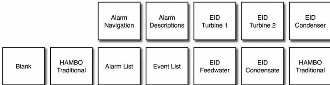
Figure 2: LCD panel layout for the turbine operator workstation in the Ecological display condition.
