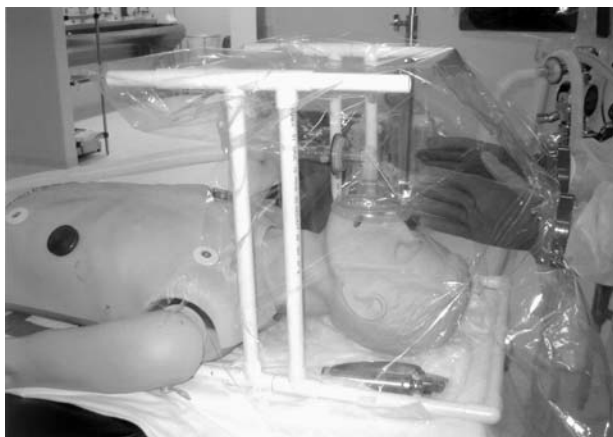
FIGURE AIR tent covering the head and the upper part of the chest of a manikin on an operating table.
